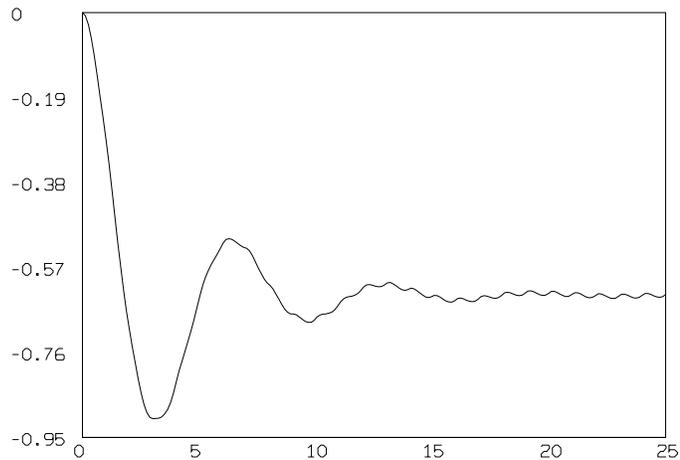
The value of the string variable ODESTR tells us what functions are numerically tabulated in the successive columns of  $M$ . The graph of the rate-of-change of the current function  $I'(t)$  can also be plotted from the data in  $M$ .
