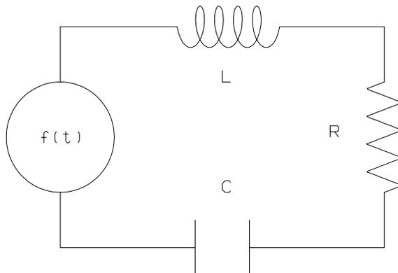
When the switch is closed at time 0, a current will begin to flow. Let  $I(t)$  be the current flowing in the circuit at time  $t$ , measured in amperes. Let  $Q(t)$  be the charge on the capacitor at time  $t$ , measured in coulombs. We have  $dQ(t)/dt = I(t)$ .
