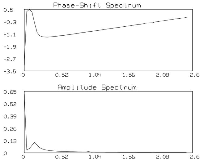
Ignoring the large DC value at frequency zero, we see that the maximum amplitude occurs at about .2 Hertz; this is the resonant frequency of the circuit. To see the amplitude spectrum at higher “resolution”, we should subtract the DC-value from our signal  $I(t)$  and compute the amplitude spectrum of this shifted signal whose mean value is now zero.
