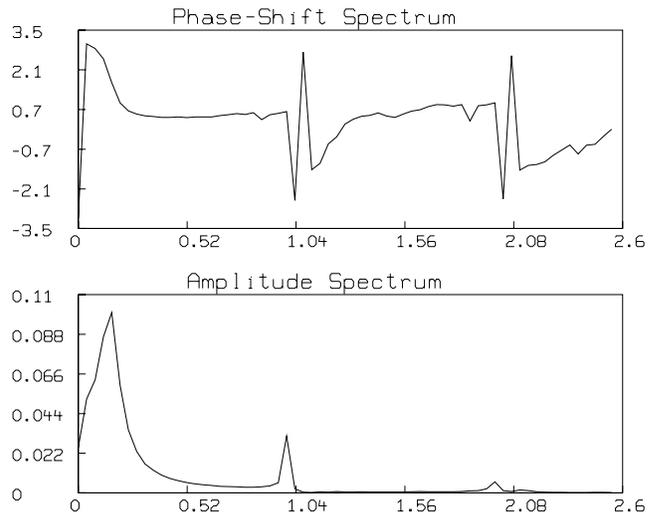
Just as before, the Fourier transform of  $I't(t)$  contains the information to construct  $I't(t)$  via its Fourier series. If the Fourier series is truncated, the resulting sum is a filtered form of  $I't(t)$  omitting the high-frequency components corresponding to the truncated terms. Below we show a graph of the Fourier series of  $I't(t)$  truncated to 7 terms, superimposed on a graph of  $I't(t)$  plotted as a dotted line.
