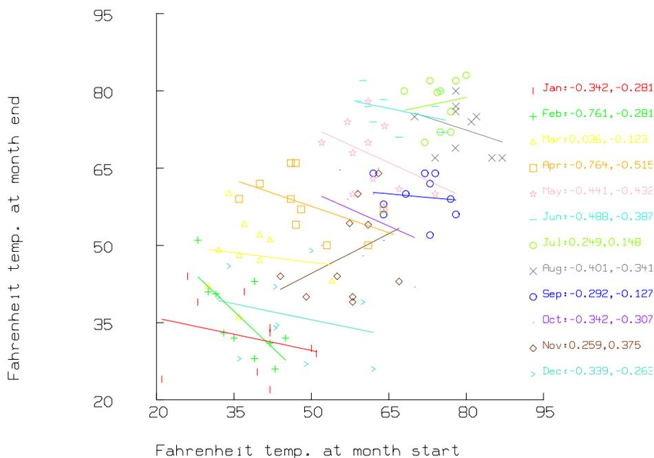
The numbers in the legend to the right side of the plot are the Spearman rank coefficient and the Pearson product-moment coefficient for each month. The line segments drawn are best-fit line-segments with colors corresponding to monthly data in the same color/symbol combination.
